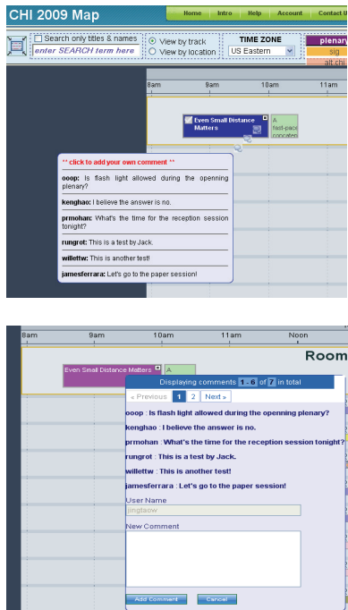
figure 4. Collaboration features in Event Maps. (top: a solid square on the top right corner indicates that there are associated comments; hovering over the indicator will display them. bottom: clicking on the indicator brings up a comment-entering widget)
