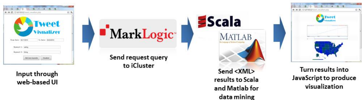
Figure 1: Overview of system design
